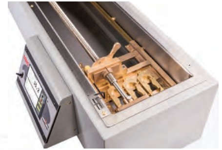
Interior of HA-1068.3F showing test molds, screw drive and disengage lever.
