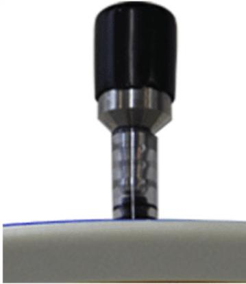
The filter self-cleaning port is connected to the sampling port, press OK twice to enter the measurement interface, open the sampling and clear the instrument self-cleaning.
