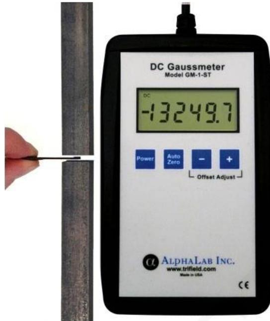
Shown measuring a strong field in a gap magnet.
