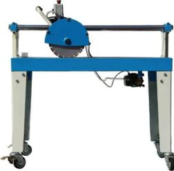
A blue industrial machine with a circular component on top, mounted on a silver metal frame with four legs and casters. | B010310030101 | Dimensiones (cm): 170x60x130 Fuente de alimentación: 380 V 50-60 Hz, 3 ph | B010310030101 |
