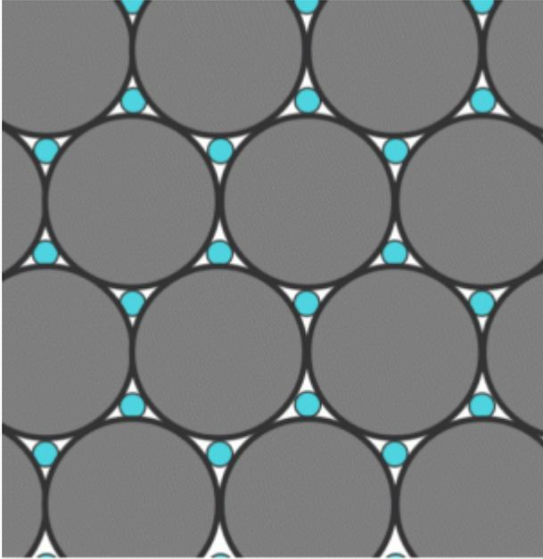
In the dry condition, the polymer elastomer does not expand, and the airway between the PE filter remains high permeability.
