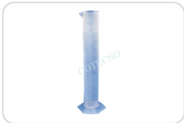
**Probeta graduada , base hexagonal 250 ml**
