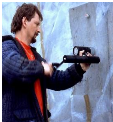
Testing the curing conditions of the "peel" protecting the reinforcement, Great Belt Link project, Denmark
