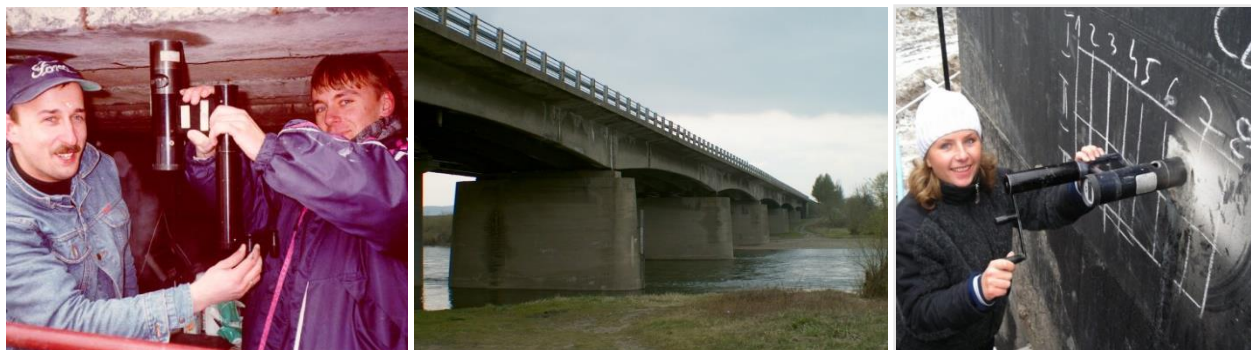
Strength evaluation of 15 bridges (25 to 52 years old) on carbonated concrete, Poland
